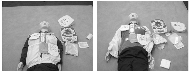
Figure 4. Electrode pads placed over jacket (left) and shirt (right) with Zoll AED.
