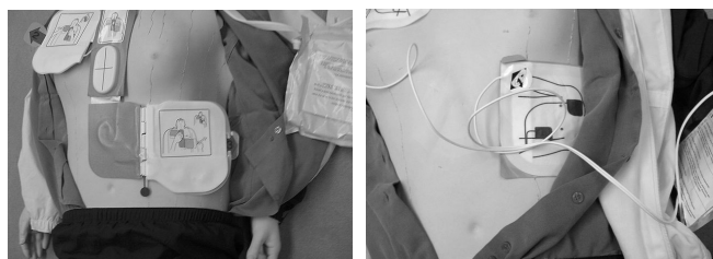
Figure 3. Electrode pad backing not removed during use of Zoll (left) and Cardiac Science (right) AEDs.
